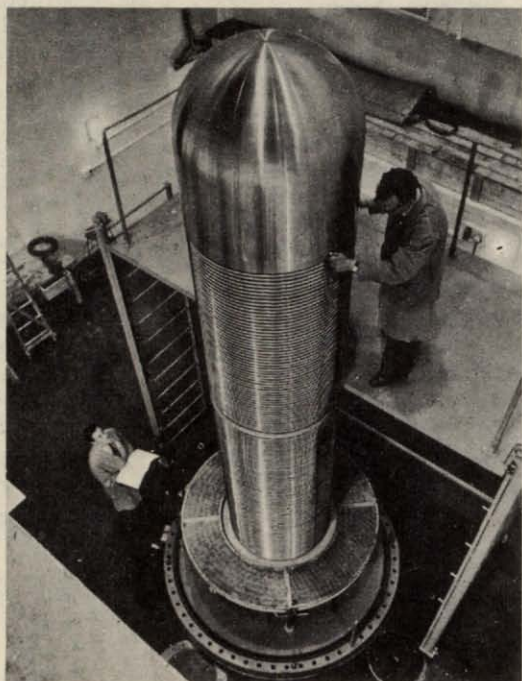
FIG. 30.10. Van de Graaff Electrostatic Generator at Aldermaston, England. The dome is the high-voltage terminal. The insulated rings are equipotentials, and provide a uniform potential gradient down the column. Beams of protons or deuterons, produced in the dome, are accelerated down the column to bombard different materials at the bottom, thereby producing nuclear reactions which can be studied.
